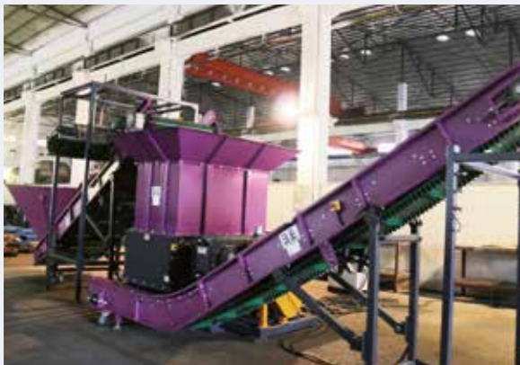
单轴粉碎机WTF40120 配磁选生产线 Single shaft shredder WTF40120 with Magnetic separation
