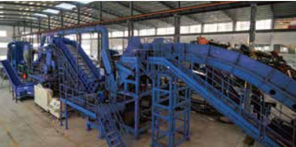
废旧金属回收线 Scrap metal recycling line 10000 kg/h
