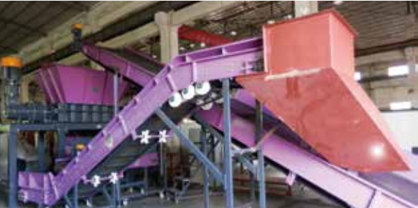
轮胎撕碎回收线 Waste tire shredding line 3000 kg/h
