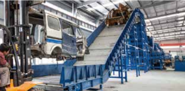
报废汽车车身回收线 Car shell crushing & recycling line 3000 kg/h
